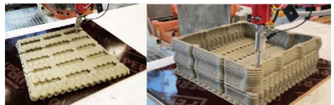
Fig. 9 Images of the printing process
