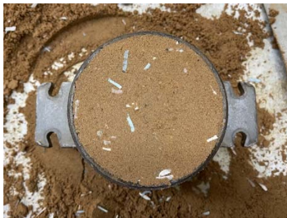
Fig. 6 Compacted sand at the optimum fiber content
