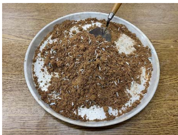
Fig. 4 Sand mixed with a 15 mm fiber content of 0.2%
