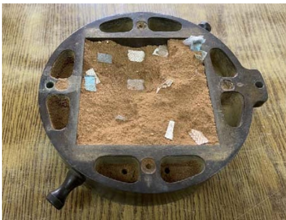
Fig. 10 Sheared sample reinforced with mask chips
