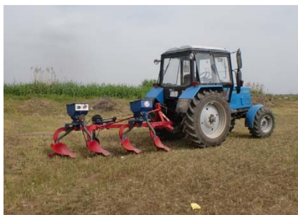
Fig. 1 General view of the combined plough
