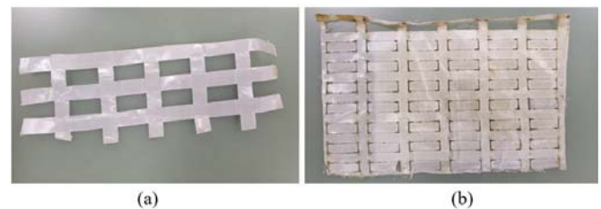
Fig. 11 100 Hour UV aged HB-210 (a) and HB-212 (b)
