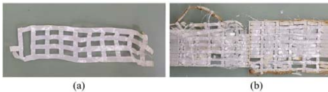
Fig. 13 800 Hour UV aged HB-210 (a) and HB-212 (b)
