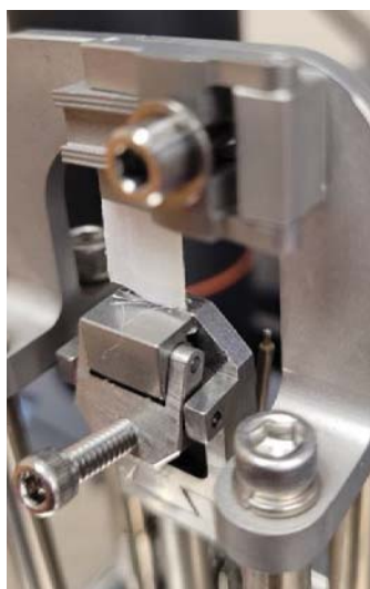
Fig. 3 DMA Film Tension Clamp with a Dyneema® HB-210 Sample Mounted
