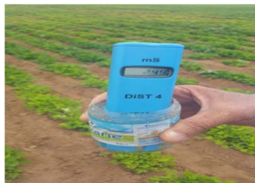
Fig. 4 Measurement of salinity by the conductivity meter
