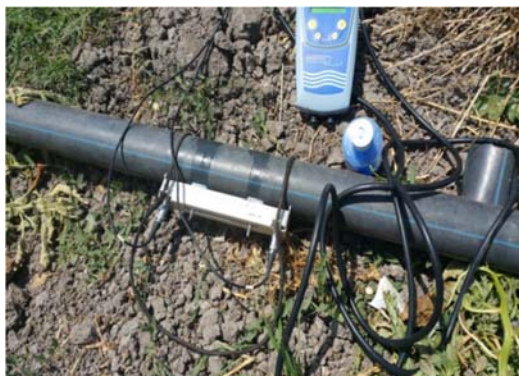
Fig. 1 Flow measurement using the Minisonic p flow meter
