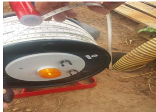
Fig. 3 Measurement of the depth of drilling by piezometric probe
