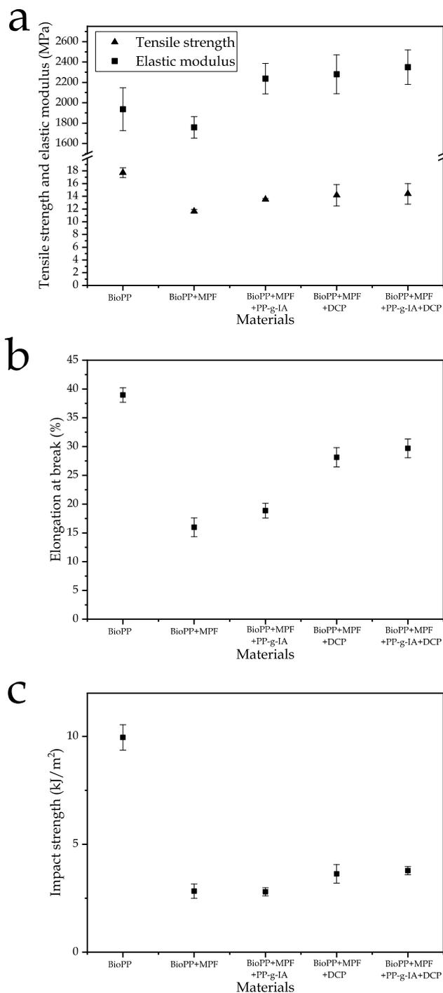
Fig. 1 Mechanical properties of the BioPP+MPF composites: (a) tensile strength and elastic modulus; (b) elongation at break; (c) impact strength
