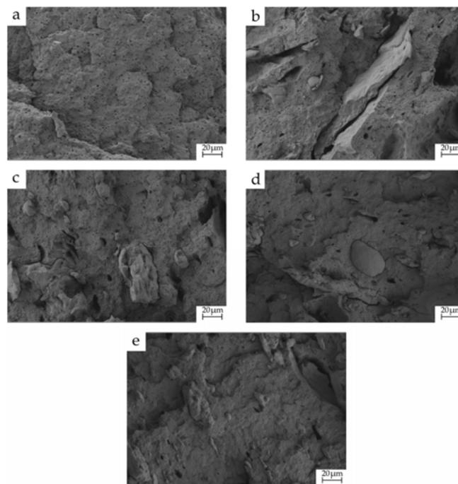
Fig. 2 FESEM images of the BioPP+MPF composites: (a) BioPP; (b) BioPP+MPF; (c) BioPP+MPF+PP-g-IA; (d) BioPP+MPF+DCP; (e) BioPP+MPF+PP-g-IA+DCP
