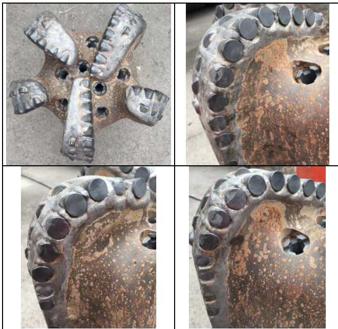
Fig. 7 Photos after the drill bit was tripped out of the well
