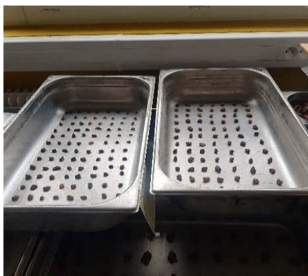
Fig. 4 Individual characterisation of the real density and water absorption of grain sizes larger than 5 mm, Arrangement in stainless steel bins (grain size class 8-10)
