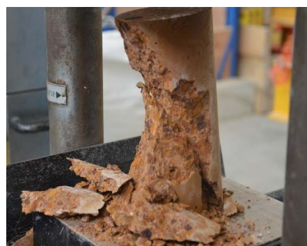
Fig. 11 Appearance of washed laterite concrete and its mode of failure in compression
