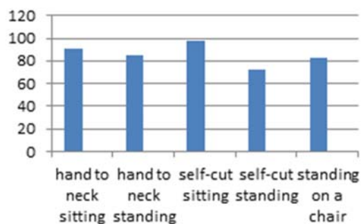
Fig. 5 Classification rates in real time using SVM algorithm to classify each gesture
