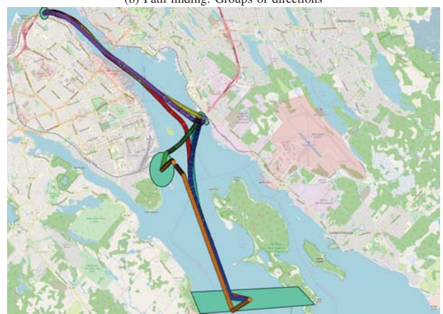
Fig. 9 A depiction of the SPTCLUST framework results of AIS cargo vessel trajectory data clustering and the extraction of its navigable routes
