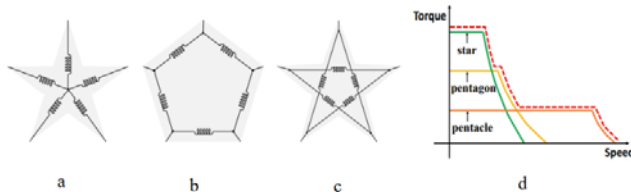
Fig. 2 Stator winding configurations for a machine with five phases: star (a), pentagon (b), pentacle (c) and corresponding torque-speed characteristics (d)
