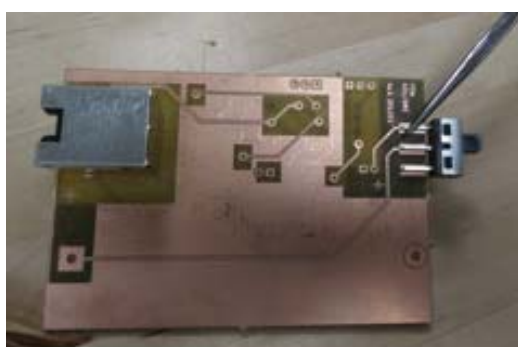
Fig. 9 Partly assembled controller board
