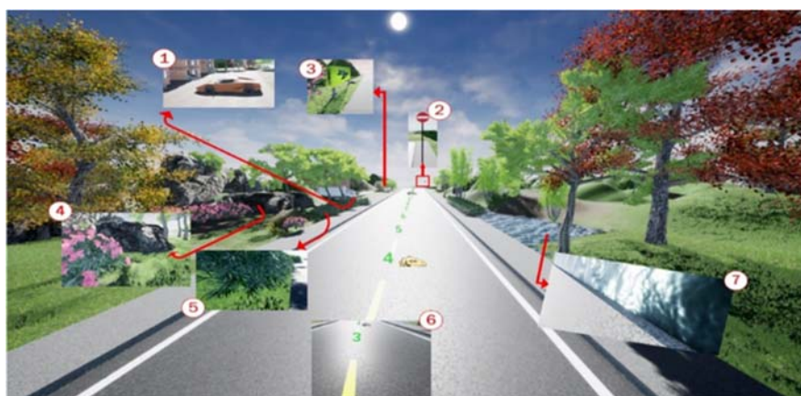
Fig. 1 Map of the test facility developed within Unreal Engine. The diagram shows a test track for one traffic sign. All the traffic signs are independently arranged in parallel in a non-occluding fashion. High fidelity environment with real-time ray tracing simulating shadows and reflection. Fine details like objects, 1) cars and buildings, 2) traffic signs at the end of the road, 3) holdings, 4) detailed rocks and vegetation with shadows, 5) realistic vegetation, 6) tarmac-like material for the road with lane markings and, 7) water reflecting sun rays
