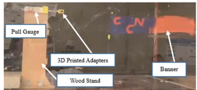
Fig. 2 Wind Tunnel Experimental Setup
