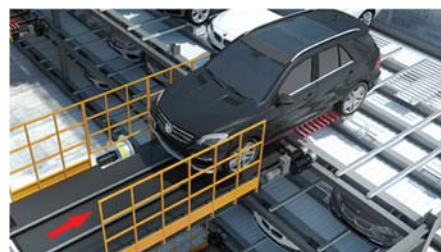
Step 5: The conveyor returns to the shuttle to complete the storage procedure.
