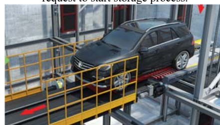
Step 3: The lift transfers the vehicle to a parking level. The dolly transfers the vehicle on to a sliding shuttle dedicated for each parking level.
