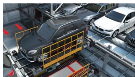
Step 4: The shuttle travels to a vacant space and the conveyor transfers the vehicle to the parking space.
