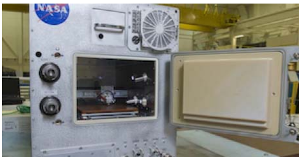
Fig. 7 Nasa's 3-D Printing Machine "Refabricator" [10]
