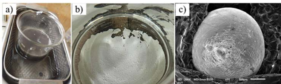
Fig. 11 Ag recovery; (a) ultrasonic leaching, (b) precipitation of AgCl and (c) Ag metal#
