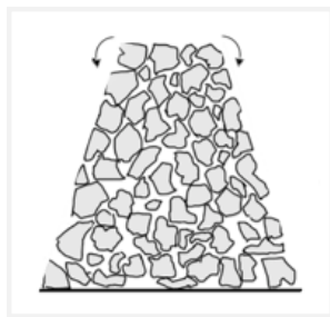
Fig. 6 Cone shape suggested by ASTM C128 for determining SSD state
