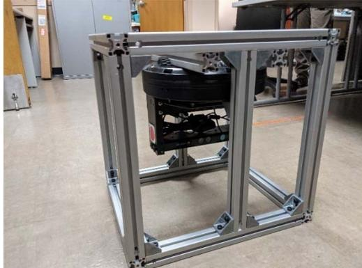
Fig. 19 6-DOF Transfer Alignment fixture
