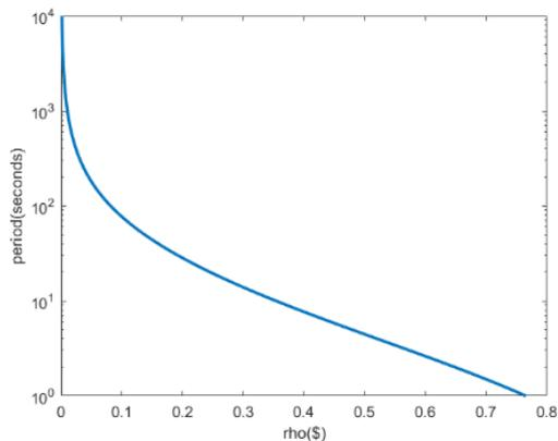
Fig. 7 Period versus reactivity insertion using reactivity equations
