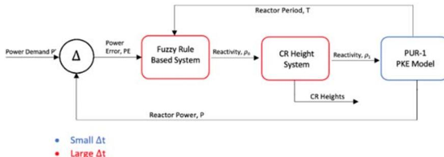
Fig. 3 Fuzzy Logic Control Loop
