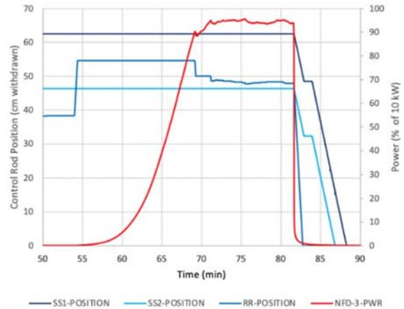
Fig. 9 Experimental CR positions versus power
