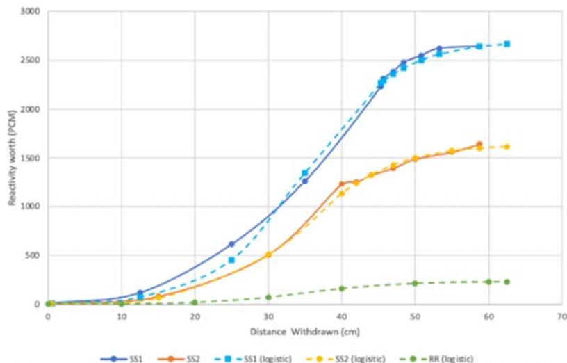
Fig. 12 Measured rod worth (Smooth lines) and Fuzzy Simulated (logistic) rod worth curves
