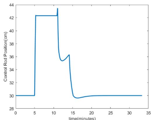
Fig. 14 CR height profile during reactor startup
