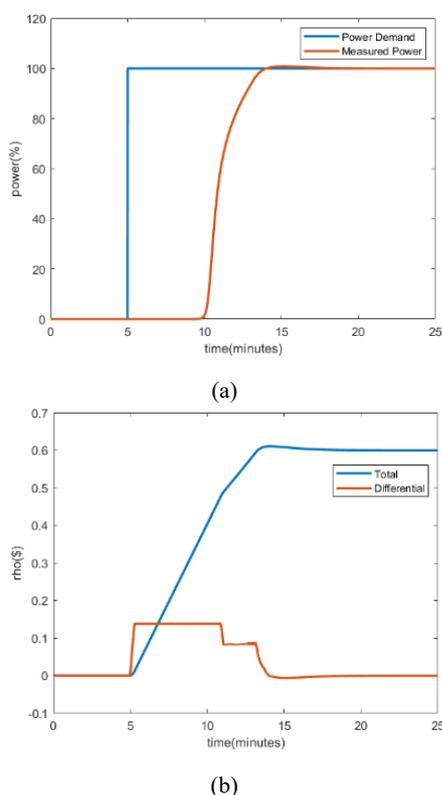
Fig. 13 Power (a) and reactivity insertion, (b) during reactor startup
