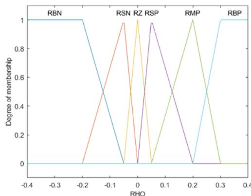
Fig. 6 Fuzzy sets for reactivity insertion (in \$): RBN (Reactivity Big Negative); RSN (Reactivity Small Negative); RZ (Reactivity Zero); RSP (Reactivity Small Positive); RMP (Reactivity Medium Positive); RBP (Reactivity Big Positive)
