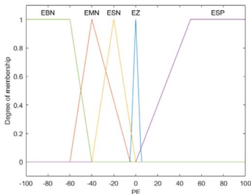
Fig. 4 Fuzzy sets for power error: EBN (Error Big Negative); EMN (Error Medium Negative); ESN (Error Small Negative); EZ (Error Zero); ESP (Error Small Positive)
