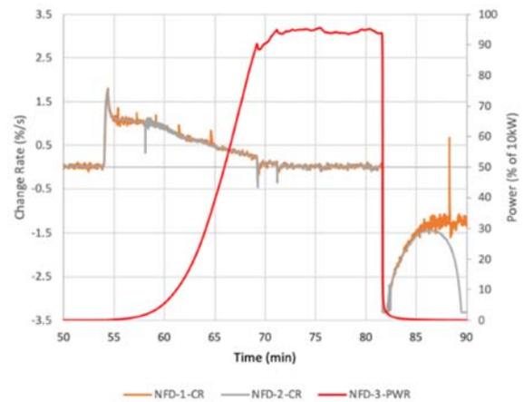
Fig. 10 Experimental power change rate versus power
