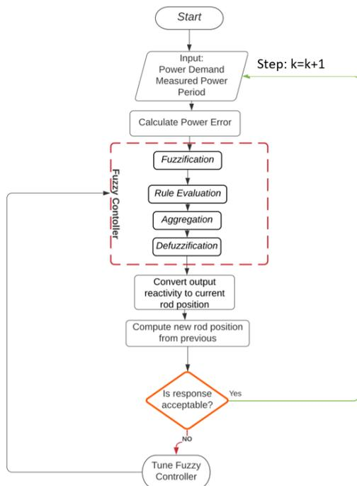
Fig. 11 Automatic CR System Algorithm
