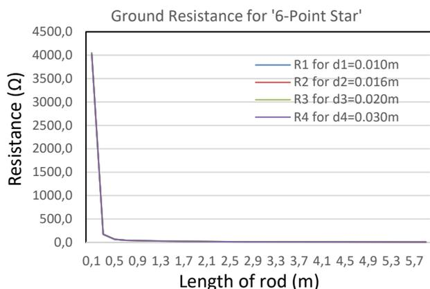
Fig. 6 The ground resistance of Six-Point Star for diameter electrode of 0.010 m, 0.016 m, 0.020 m, and 0.030 m with soil resistivity of 100 Ωm
