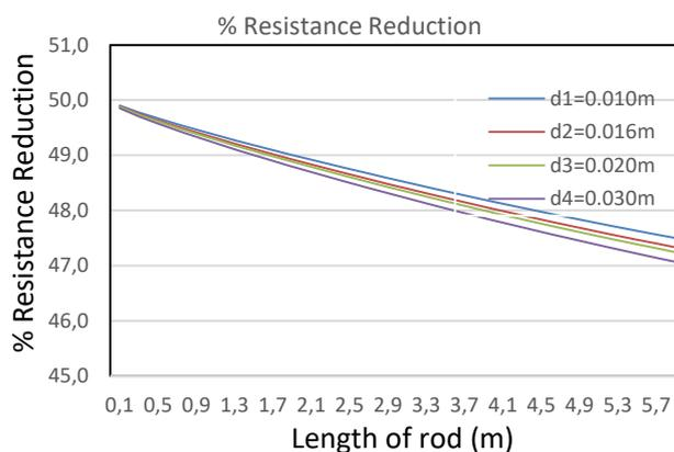
Fig. 4 Percentage reduction between Single Ground Rod and Two Ground Rod
