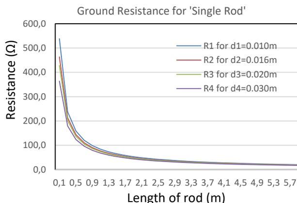
Fig. 2 The ground resistance of Single Ground Rod for diameter rods of 0.010 m, 0.016 m, 0.020 m, and 0.030 m respectively with soil resistivity of  $100 \Omega\text{m}$
