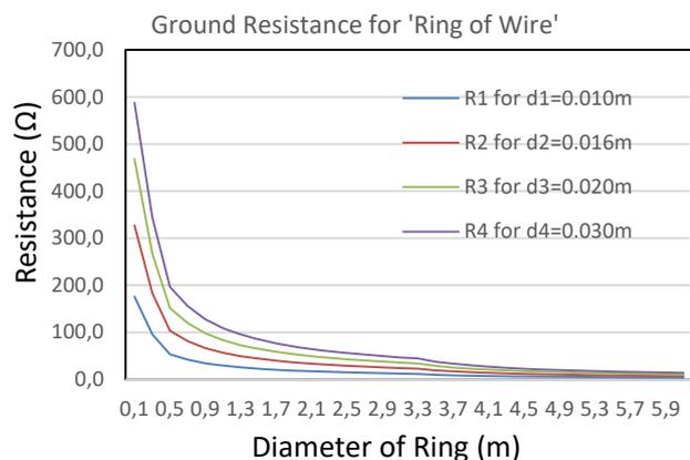
Fig. 8 The ground resistance of Ring of Wire for diameter rods of 0.010 m, 0.016 m, 0.020 m, and 0.030 m with soil resistivity of 100  $\Omega$ m
