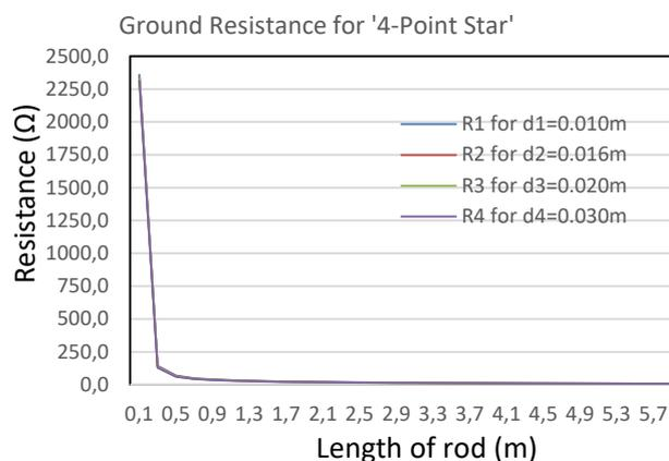
Fig. 5 The ground resistance of Four Point Star for diameter rods of 0.010 m, 0.016 m, 0.020 m, and 0.030 m respectively with soil resistivity of 100  $\Omega$ m and at depth level 0.5 m from the ground surface
