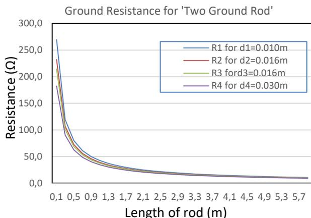
Fig. 3 The ground resistance of Two-Ground Rod for diameter rods of 0.010m, 0.016 m, 0.020 m, and 0.030 m with soil resistivity of 100  $\Omega$ m
