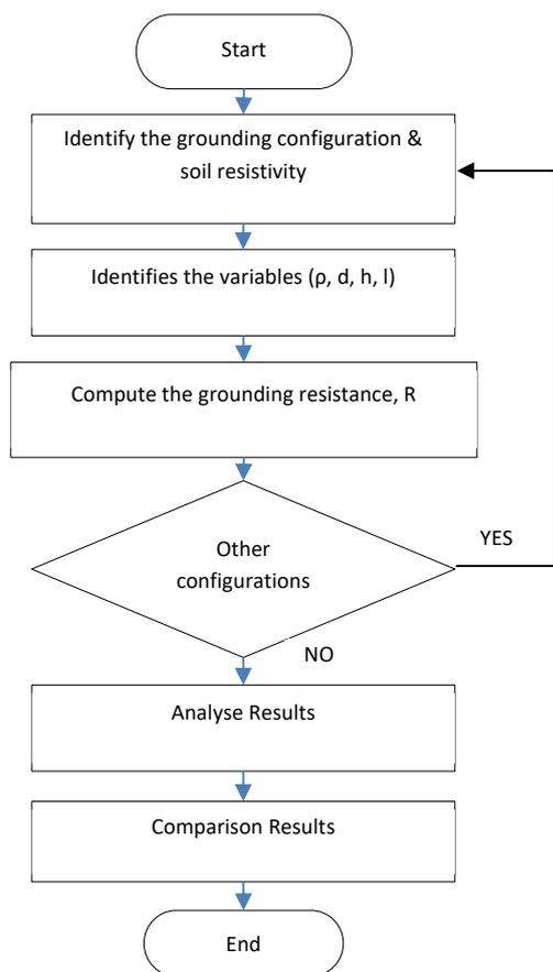
Fig. 1 Analysis procedure for grounding technique
