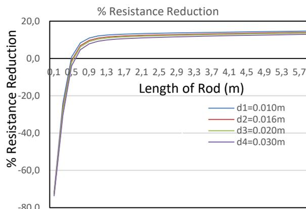
Fig. 7 Percentage reduction (Resistance coefficient) between Four-Point Star and Six Point Star
