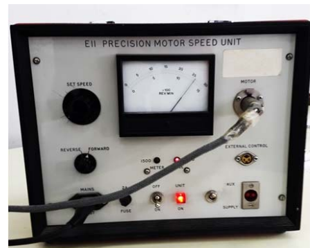
Fig. 3 The driver of synchronous motor to increase rotation speed
