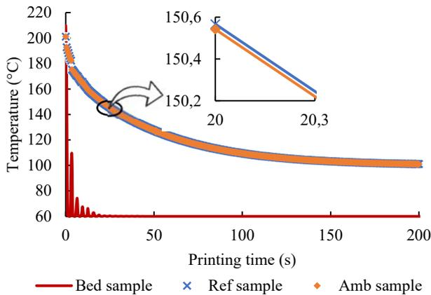
Fig. 1 Overall cooling of element m (top layer) after deposition in ref, amb, and bed sample. An inset plot is presented to show the difference in the cooling curve between sample ref and amb is magnified at 20 s of their print time
