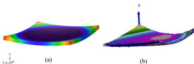
Fig. 5 Comparison of the simulated and 3D scanned warpage of bed sample
