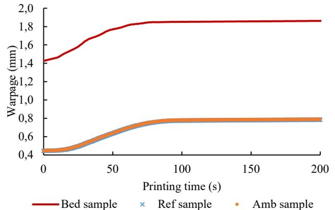
Fig. 3 Element m warpage from ref, amb and bed sample plotted against their overall printing time
