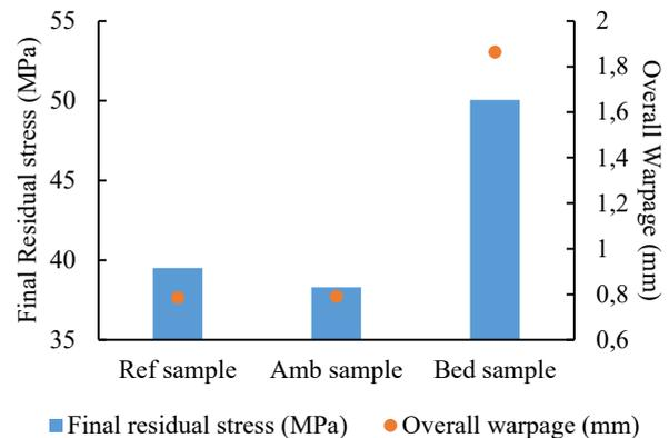
Fig. 4 Final residual stress of element m from ref, amb and bed sample against the overall warpage with respect to their printing condition
