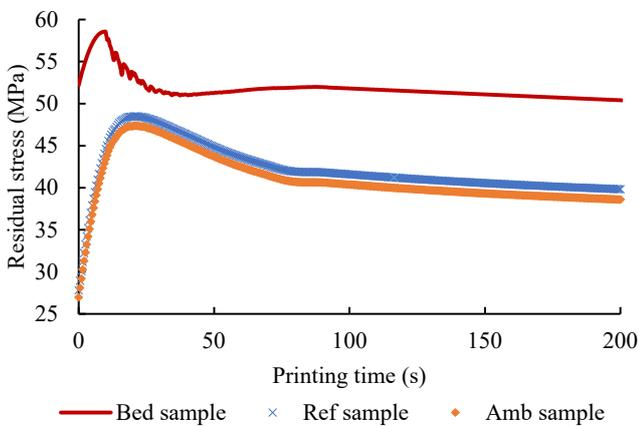
Fig. 2 Built-in residual stress of element m from ref, amb and bed sample plotted against the overall printing time
