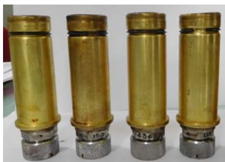
Fig. 6 (a) Front view of gas generator after firing
