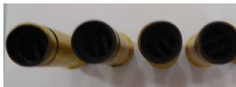
Fig. 6 (b) Top view of gas generators after firing
