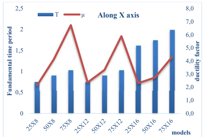
Fig. 8 Relation between fundamental time period and ductility factor for 16, 12 and 8 story buildings with steel V bracings along the X direction
