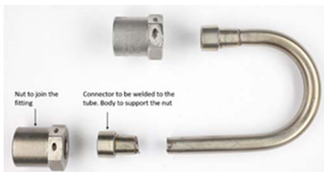
Fig. 1 (c) general view of the fractured tube as received
