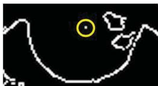
Fig. 14 The iris's center point calculated using the Hough transform
