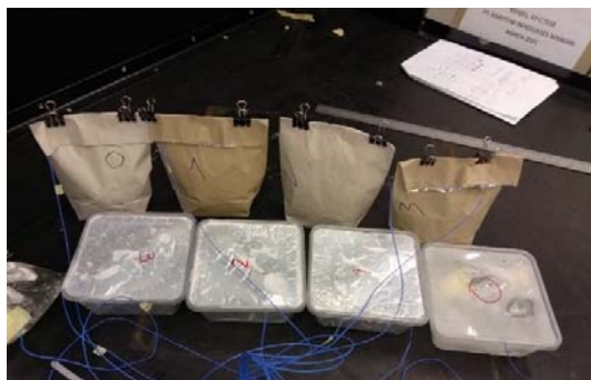
Fig. 3 Example of the measurement setup of the food packages made of food paper and plastic boxes, with and without aluminum foil
