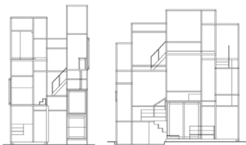
Fig. 14 Sections of Fujimoto's House NA, showing spatial heterogeneity and homogeneity
