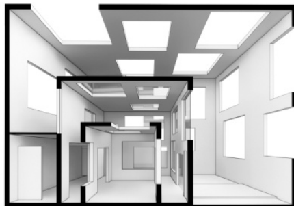
Fig. 10 3D section of Fujimoto's House N, showing the idea of a house inside a house inside a house
