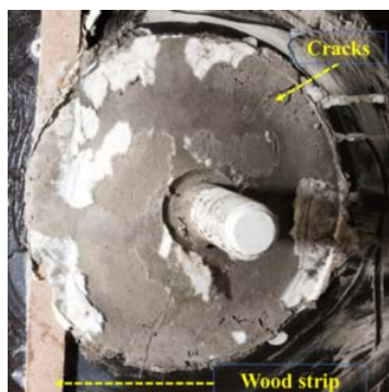
Fig. 13 Effect of uneven surface on the distribution of mortar under the dome-plate
