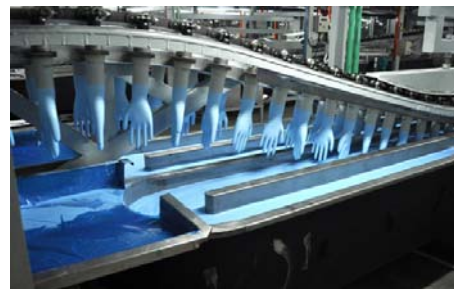
Fig. 1 Latex-dipping process in a production line
