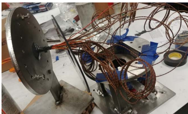
Fig. 1 Test apparatus with Celmet and silicon powder just before sealing. From left to right: lid, Viton™ gasket surrounding thermocouples, flange, 1000 cm 3 chamber with flange
