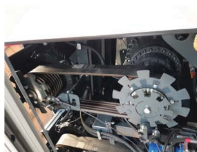
Fig. 4. Incremental encoder sensors on the shredder, mounted on the motor and rotor.
