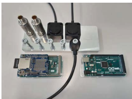
Fig. 2. Arduino datalogger for accelerations and motor parameters recording.
