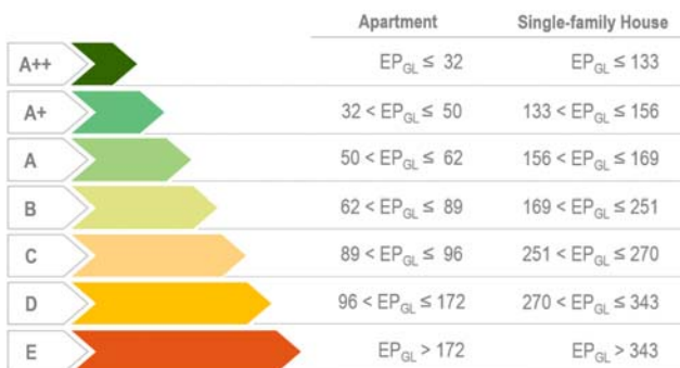
Fig. 2 Energy classification scales of the two case studies (apartment in multi-story building, on the left, single-family house, on the right) situated in the same climate zone
