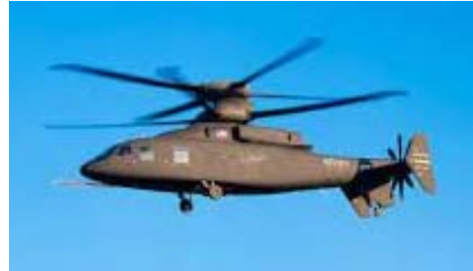
Fig. 2 Sikorsky-Boeing SB-1 Defiant in flight with dual rotors and tail prop [33]
