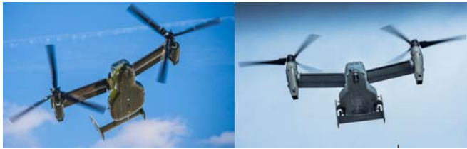
Fig. 1 The V-22 Osprey can switch between flying like an airplane or a helicopter during any flight. The V-22 Osprey is pictured on the left flying horizontally with the tiltrotor in a forward motion direction and in the adjacent photo on the right the same aircraft flies vertically with the tiltrotor in a lift configuration [18]
