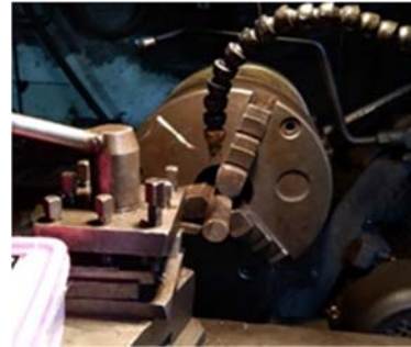
Fig. 2 Experimental set up for EN3 turning
