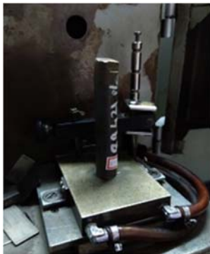
Fig. 1 Spectrometer setup for chemical composition test
