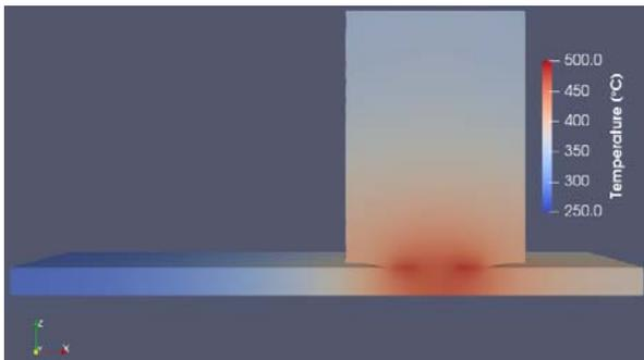
Fig. 3 Temperature distribution in the system, under 3000 rpm and 465 N during 500 s
