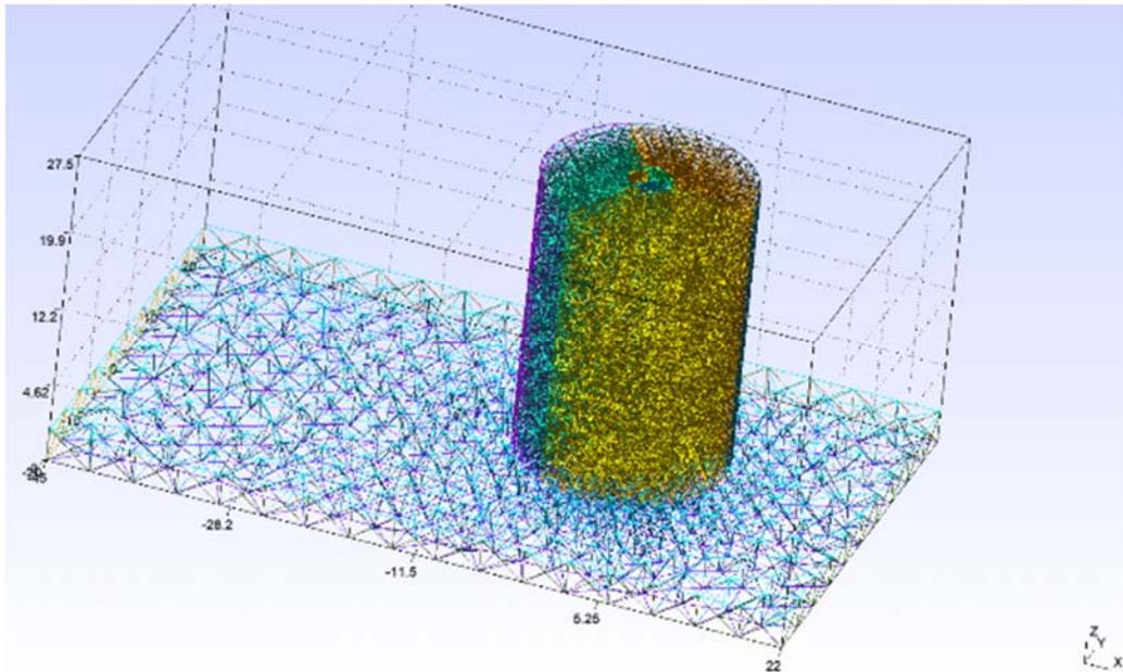
Fig. 2 Meshing of the system on GMSH
