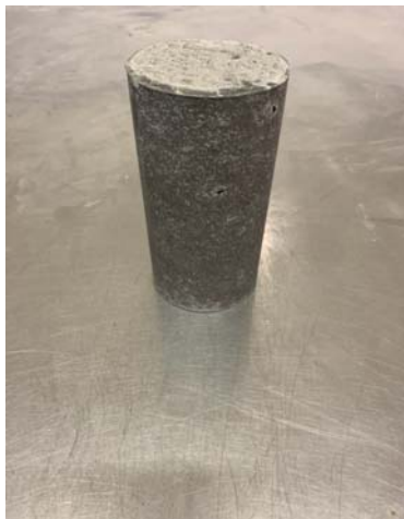
Fig. 6 Dry Mix Cylinder with imperfections
