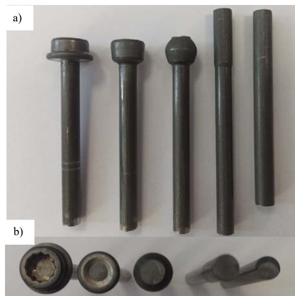
Fig. 1 Successive steps of multi-stage forging a bolt, (a) side view in the Z axis, (b) upper view in the Y axis
