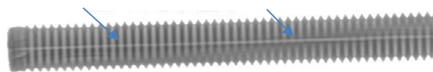
Fig. 2 X-ray image of the defective threaded bolt pin with visible non-metallic inclusion
