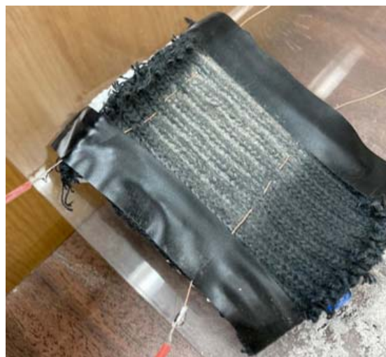
Fig. 6 Lunar dust simulant on the fabric with an electrode distance of 5 cm after applying the ECS but prior to brushing
