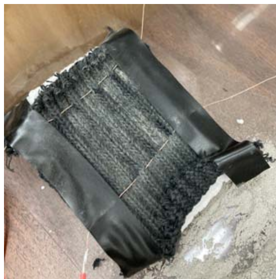
Fig. 7 Lunar dust simulant on the fabric with an electrode distance of 5 cm, after the brushing (end of dust removal process)
