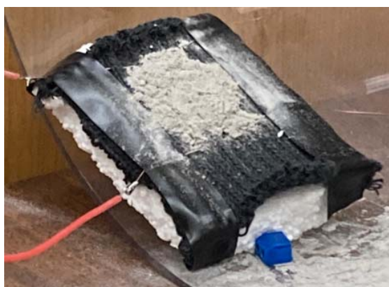
Fig. 5 Lunar dust simulant on the fabric for the electrode distance of 5 cm, prior generating the electrostatic force
