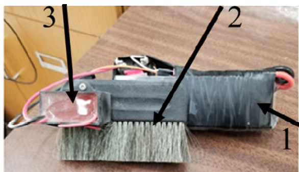
Fig. 2 Components of the Thunderon brush: (1) Power supply; (2) Thunderon brush; (3) Ion generator
