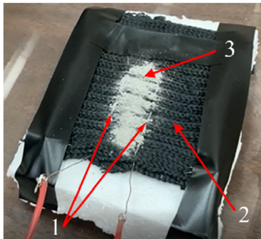
Fig. 1 Components of the fabric: (1) Electrodes; (2) Kevlar fabric; (3) Lunar dust simulant
