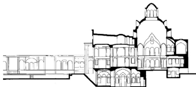
Fig. 8 Section of Borujerdi house, elaborating the height and placement of skylight holes [33]
