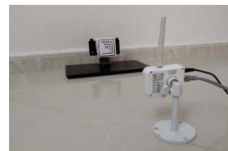
(c) Distance and Viewing Angle Test Dispositive
