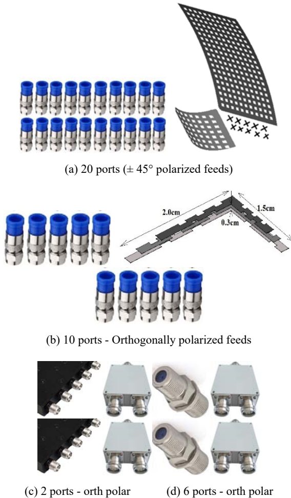
Fig. 9 Two rows of feeds generating 10 beams combined into different configurations of ports
