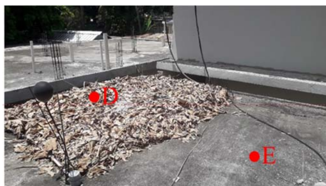
Fig. 4 Photograph of the roof in Haiti where the experiment was carried out, one part covered (D) with banana leaves and the other part not covered (E). The roof was subjected to the influence of solar radiation in order to test the thermal performance of banana leaves. In fact, the temperature of the bare concrete and that of the covered concrete has been measured. Tsenc: outside surface temperature of bare concrete (E), i.e., not covered with banana leaves. Tsec: outside surface temperature of the concrete covered (D) with banana leaves, i.e., under the banana leaves
