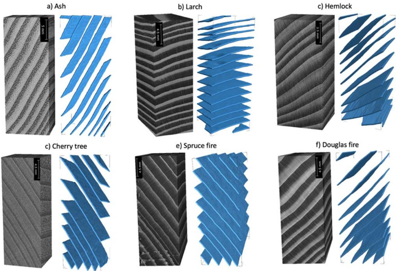
Fig. 3 The measured X-CT image stack and their calculated 3D tree-ring surfaces (plots in blue) for each wood specie studied
