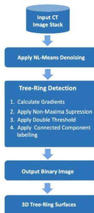
Fig. 1 The pipeline overview of the proposed approach
