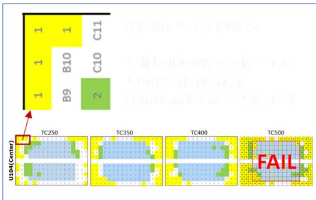
Fig. 10 Cumulative Ball Crack Analysis
