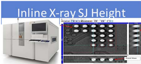
Fig. 6 Inline X-Ray Solder Joint Height Analysis
