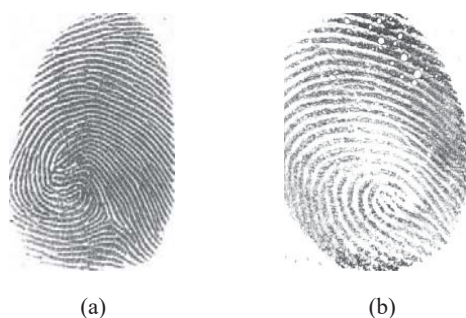
Fig. 1 Image of a spoof fingerprint made out of gelatine (a) and a live fingerprint (b)
