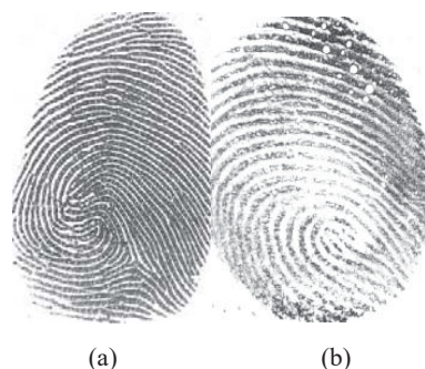
Fig. 1 Image of a spoof fingerprint made out of gelatine (a) and a live fingerprint (b)
