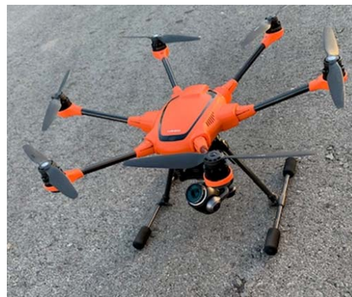
Fig. 5 Drone applied to capture images
