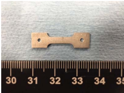
Fig. 4 Representative tensile specimens extracted from the ECAP magnesium billet
